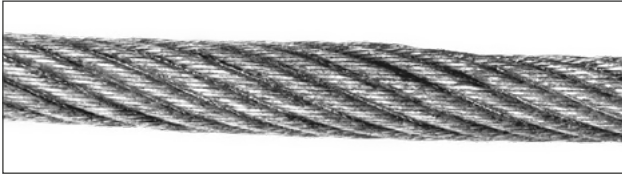
Fig.: Local increase in rope diameter due to deformation of the core
