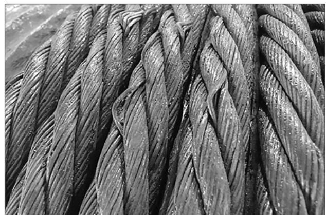
Fig.: Protruding wire loop
