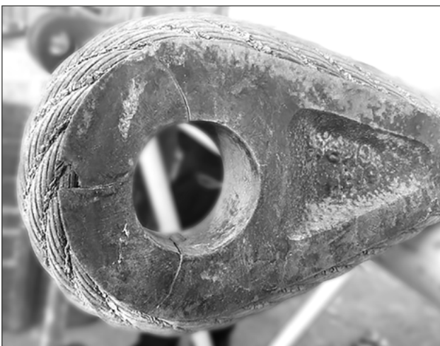
Fig.: Cracks in a solid thimble
