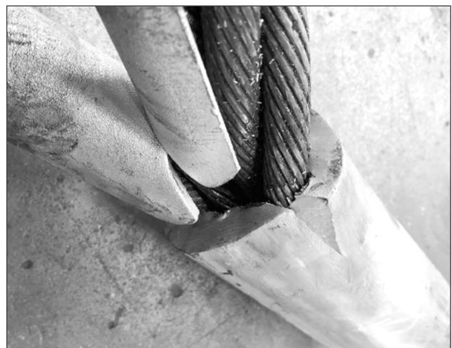
Fig.: Crack in the swaging area of an aluminum ferrule
