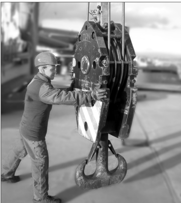
Fig.: Turning the hook block into its neutral position
