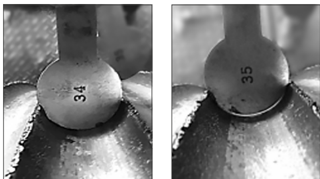
Fig.: Reduced groove diameter on a drum
