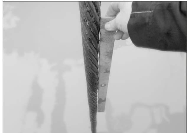
Fig.: Measurement of waviness
