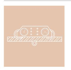
Tension Measuring ensures that the ropes are using even tensions. This is of paramount importance in applications where multiple ropes are being used for hoisting.
